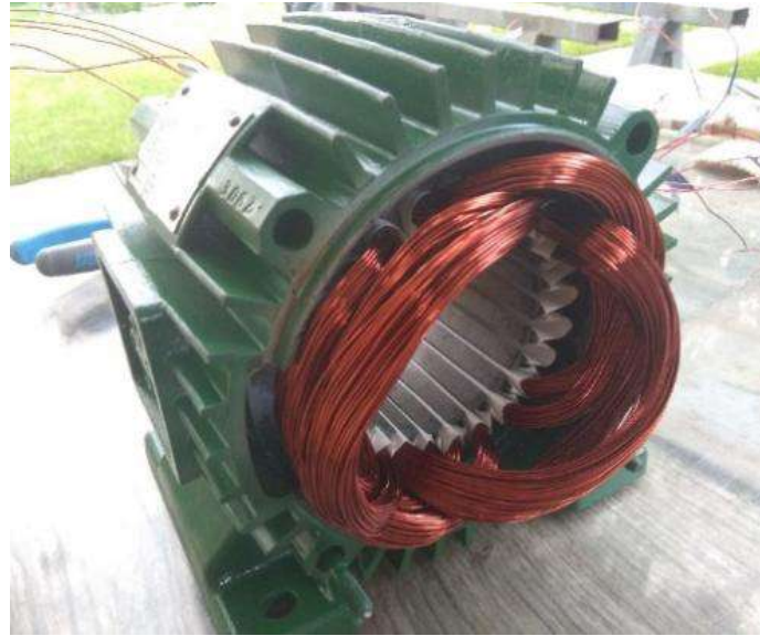
Figure 2.4 Rewinding 3-Phase Motor (Source: https://www.instructables.com/Rewinding-3-Phase-Motor/ )
