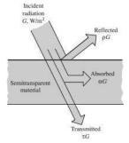
G<sub>abs</sub>, G<sub>ref</sub>, and G<sub>tr</sub> are the absorbed, reflected, and transmitted portions of it, respectively.
