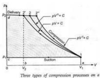
Three types of compression processes on a p-V diagram
